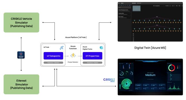
Network IDS for MITM Attack Detection [EV - EVSE CSMS Based] Feeding DT
